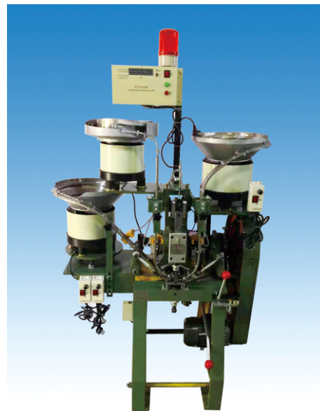
NKJX018 Three-Railways & vibrating Discs Assembled Button Machine Speed: 9600Pcs/H Power: 0.37KW/380V/50HZ Size: 1080*600*1060mm Weight: 320Kg
